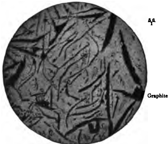
Fig. 60. Gray Cast Iron, cast in sand. Silicon, 1.54 per cent; Sulphur, 0.075 per cent (Sauveur, The Metallographist , III, p. 156).
